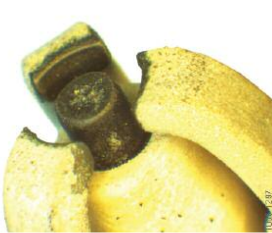
The spark plug above shows a normal wear pattern with no excessive electrode wear or insulator damage.
